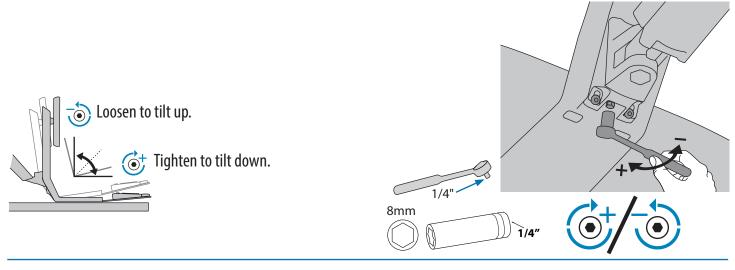
3 After desired tilt is achieved, retighten these two screws to secure.
